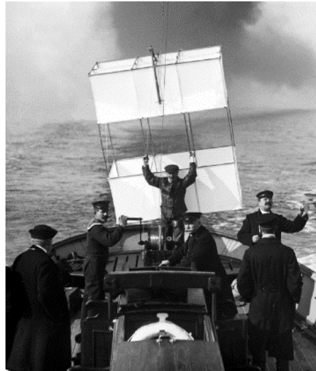
Launching of a Lindenberg N-kite on the Rovuma river in 1908 during the German expedition for the exploration of the upper air in tropical East Africa
